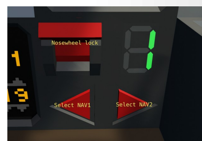
Figure 7: Pilot's nav selector and nosewheel control panel (AS10D)
